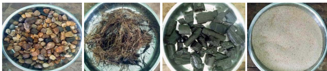
Figure 2. Gravel, fiber of toddy palm leaf, charcoal and sand for water treatment
