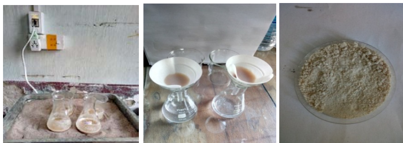
Figure 2 Extraction of chitin by deproteinization and demineralization
