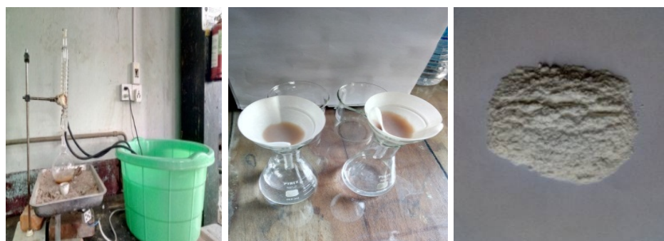
Figure 3. Extraction of chitosan by deacetylation
